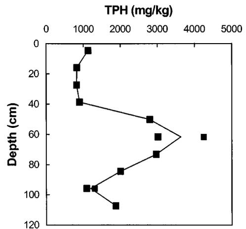
**Fig. 3.** Depth profile of total petroleum hydrocarbons in Seaplane Lagoon sediment. Multiple points for TPH at 62 and 96 cm indicate duplicate measurements.
