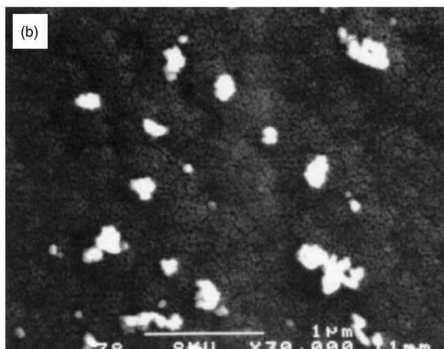
FIG. 5. SEM images of nonirradiated and irradiated NaCl particles. (a) Nonirradiated NaCl Particles from the nebulizer system. (b) NaCl particles irradiated at 0.16 J/cm 2 , 50 Hz.
