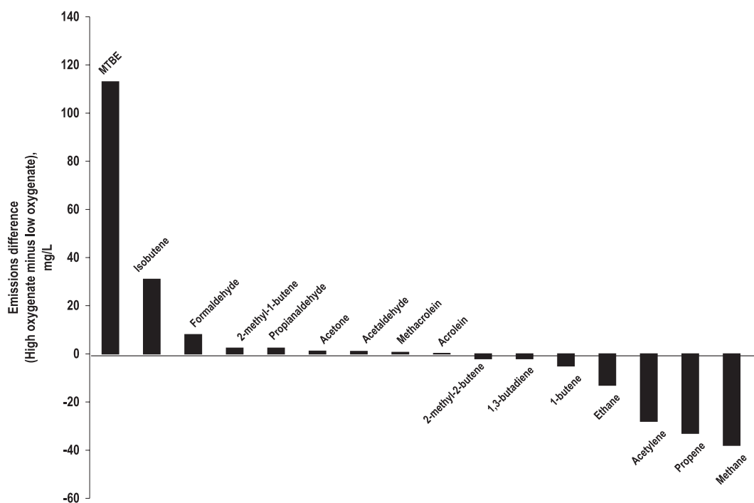
Fig. 3. Comparison of on-road emissions (Caldecott tunnel measurements) for high-oxygenate (October 1994) and low-oxygenate (August 1994) fuels. Note that both fuels are non-reformulated. Data from Kirchstetter et al. (1996). Emissions are in mg/l fuel. Again, bars above the axis indicate increases in emissions which are associated with the high-MTBE fuel compared to the low-MTBE fuel.
