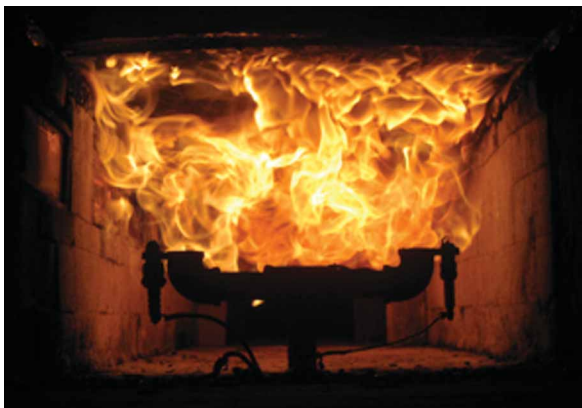
Figure 1 The Steiner Tunnel, showing the flame being applied to the ceiling. Source: Intertek Testing Services Inc, Elmendorf, TX.
